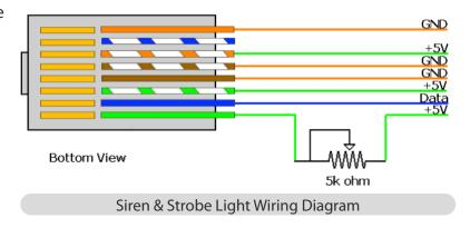
Alternatively, you can wire in a potentiometer, or a switch into the siren/strobe sensor. This would allow you to control the volume or disable the siren while leaving the strobe light active. You can wire in-line, a 5 ohm potentiometer (pot), or a switch with the siren, then it would be possible to adjust volume, or turn it on or off completely.
